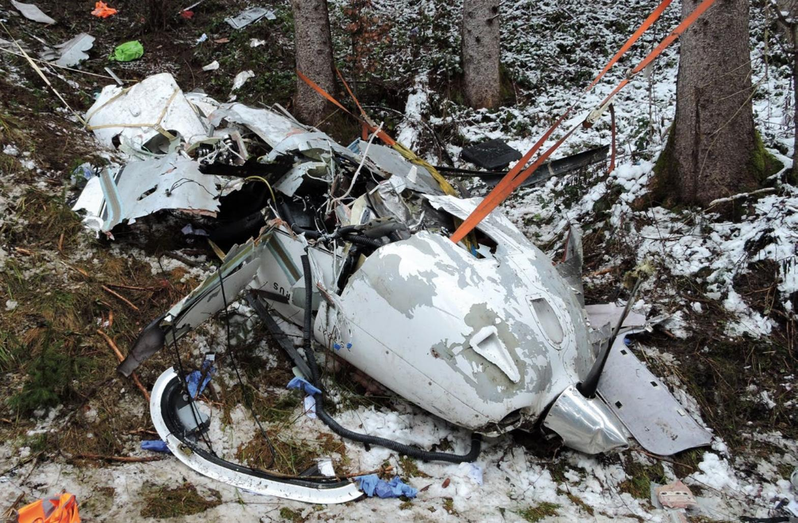
Figure 4: SR22T wreckage after CFIT.
