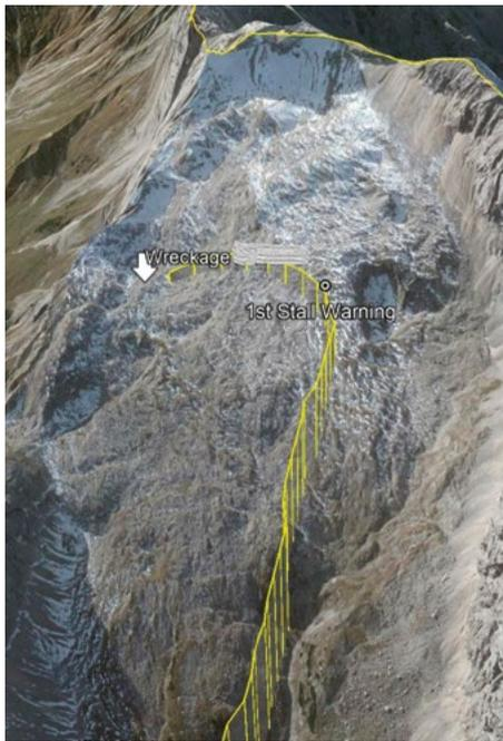
Figure 1: Final Flight Track (Source: SUB)
